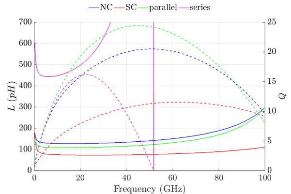
Fig. 4. Simulated equivalent inductance (solid lines) and quality factor (dashed lines) versus frequency for the transformer TS11.
