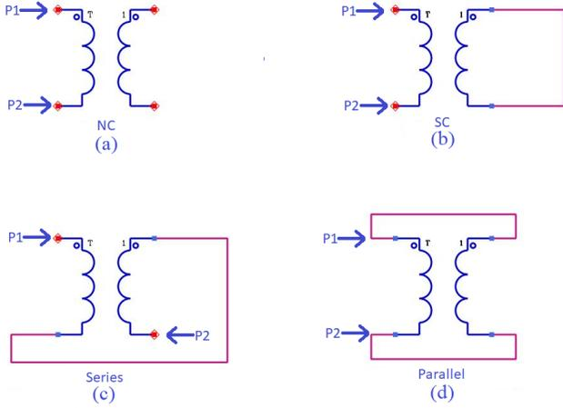
Fig. 1. Wiring topologies for different inductances: NC, (a) SC, (b) Series (c) and Parallel. (d)
