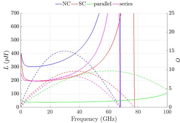
Fig. 5. Simulated equivalent inductance (solid lines) and quality factor (dashed lines) versus frequency for the transformer TS21.
