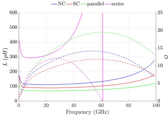
Fig. 3. Simulated equivalent inductance (solid lines) and quality factor (dashed lines) versus frequency for the transformer TP11.
